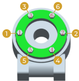
FIGURE 4. BOLT TORQUE SEQUENCE
